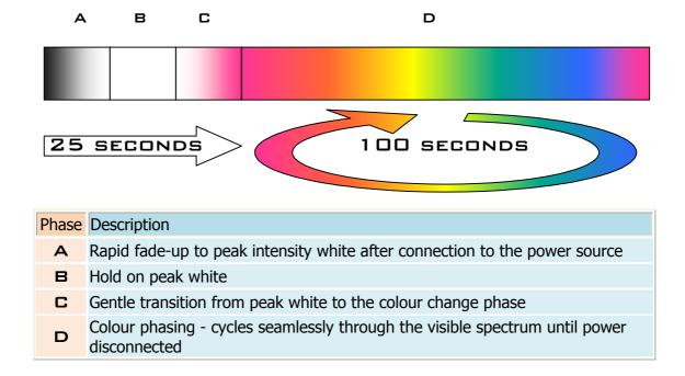
**Freezing the colour** At any time, the programme may be halted by briefly switching the power supply off then back on again (within less than a second). This simple action allows the light source to be frozen on any particular colour (or white)
